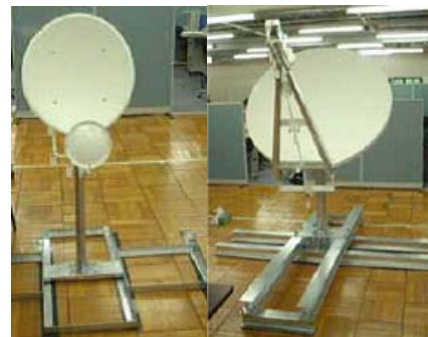
Figure 15. USAT (45 cm antenna) Figure 16. VSAT (1.2 m antenna)
