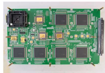
Figure 11. ATM switch core board
